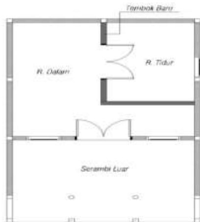
Figure 04 : Modified floor plan sketch of Taneyan Lanjhang with the addition of a bedroom.
