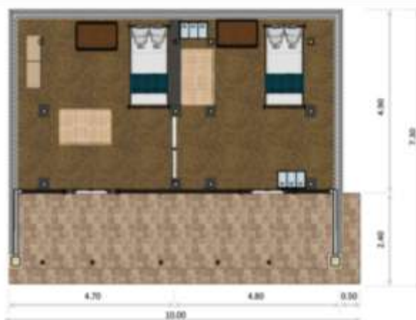
Figure 03: Sketch of a standard Taneyan Lanjhang floor plan with a relatively limited land area, with a minimum of two bedrooms and a veranda.
